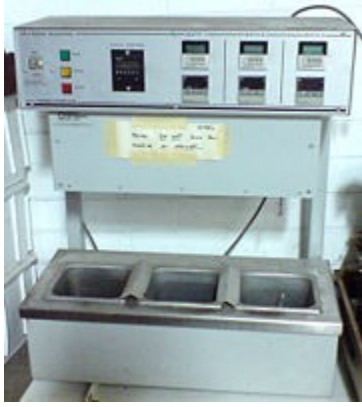
Figure 1b: A very old three-temperature thermal cycler for PCR
