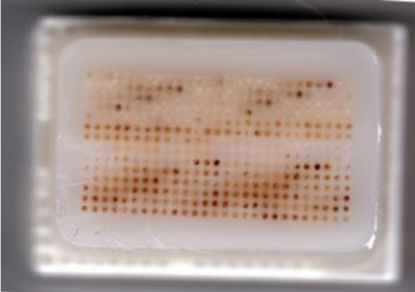
0.6um core Tissue MicroArray Block
